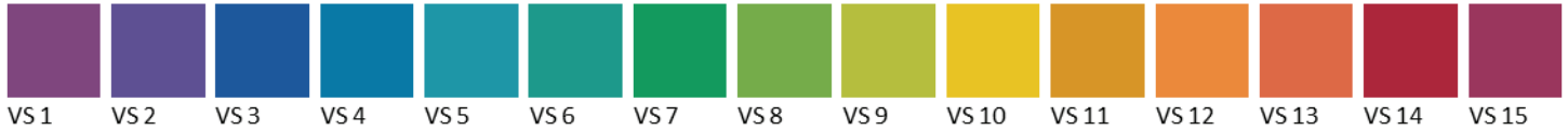
Figure 3. Approximation of color samples used for the calculation of CRI, R_9-R_{14} , and CQS. Because appearance will vary based on the illumination condition, display settings, printing properties, and/or viewing conditions, these are only examples. Adapted from NIST data.
